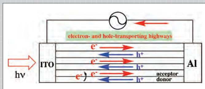
Schematic illustration of ideal bulk heterojunction solar cell
