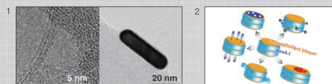
1. Electron microscopy images of photoresponsive nanomaterials. Carbon nanotubes (left) and gold nanorods (right).
