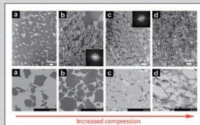
Two-dimensional (2D) assemblies of nanoscale building blocks prepared by Langmuir-Blodgett technique (top: BaCrO<sub>3</sub> nanorods, bottom: graphene oxide nanosheets)
