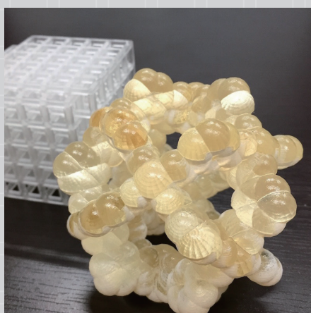
3D printed models of porous materials. Metal-organic cuboctahedron (front) and entangled metal-organic frameworks (back)
