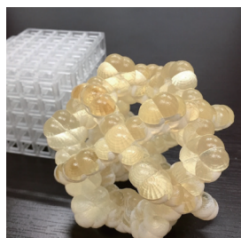
3D printed models of porous materials. Metal-organic polyhedral (MOP)(front) and entangled metal-organic frameworks (back)
