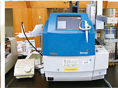
This apparatus, popular in the laboratory, is commonly called a "microwave oven." It operates on the same principles as market-available ones. In several minutes it heats liquids, which via other heat sources would take hours. Different from common microwave ovens, it is built to be explosion-proof, which means it is robust enough to prevent the container from scattering away in postulated explosions.
