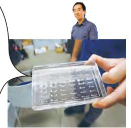
I can construct testing apparatuses myself, even if they are large. Three-dimensional printers are very useful for building testing devices because they can materialize ideas quickly, such as in the case of this cell cultivation instrument.
