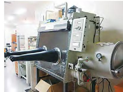
This apparatus is commonly known as a "glove box." The user places their arms into the box via the black gloves to work while ensuring that the interior is isolated from the surrounding air. The box is filled with nitrogen or another inert gas.
