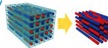
By using porous materials as a mold, this technique completely mixes the polymer at the molecular level which has not been done before
