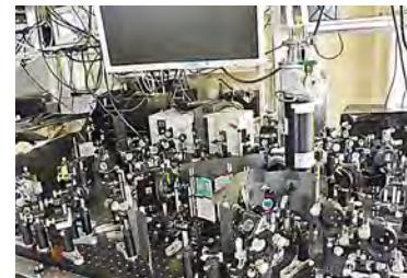
The rows of magnifying glass-like tools create a device that generates terahertz waves.
