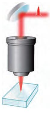
Refractive index distribution can be created inside various transparent materials with a spatial resolution of less than micrometer by focusing femtosecond laser pulses.
