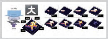
Fluorescence images of propagating excitation waves in a light-controlled path
