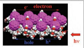
Highly efficient hole and electron transportation by molecule-level bicontinuous donor-acceptor network
