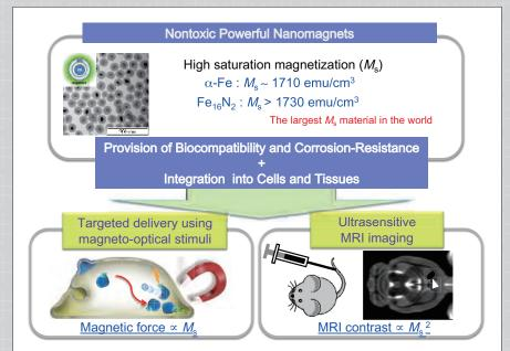
Nontoxic powerful nanomagnets prepared in our group, which are being employed for progressive applications such as spatiotemporally controlled intracellular release of physiologically active substances and ultrasensitive MRI imaging.
