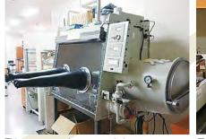
This apparatus is commonly known as a "glove box." The user places their arms into the box via the black gloves to work while ensuring that the interior is isolated from the surrounding air. The box is filled with nitrogen or another inert gas.
